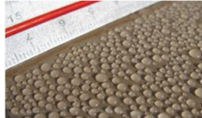
Condensation on some packing tape left on the Louvre site. The surface has a low 'wettability' and so the droplets are near spherical.
