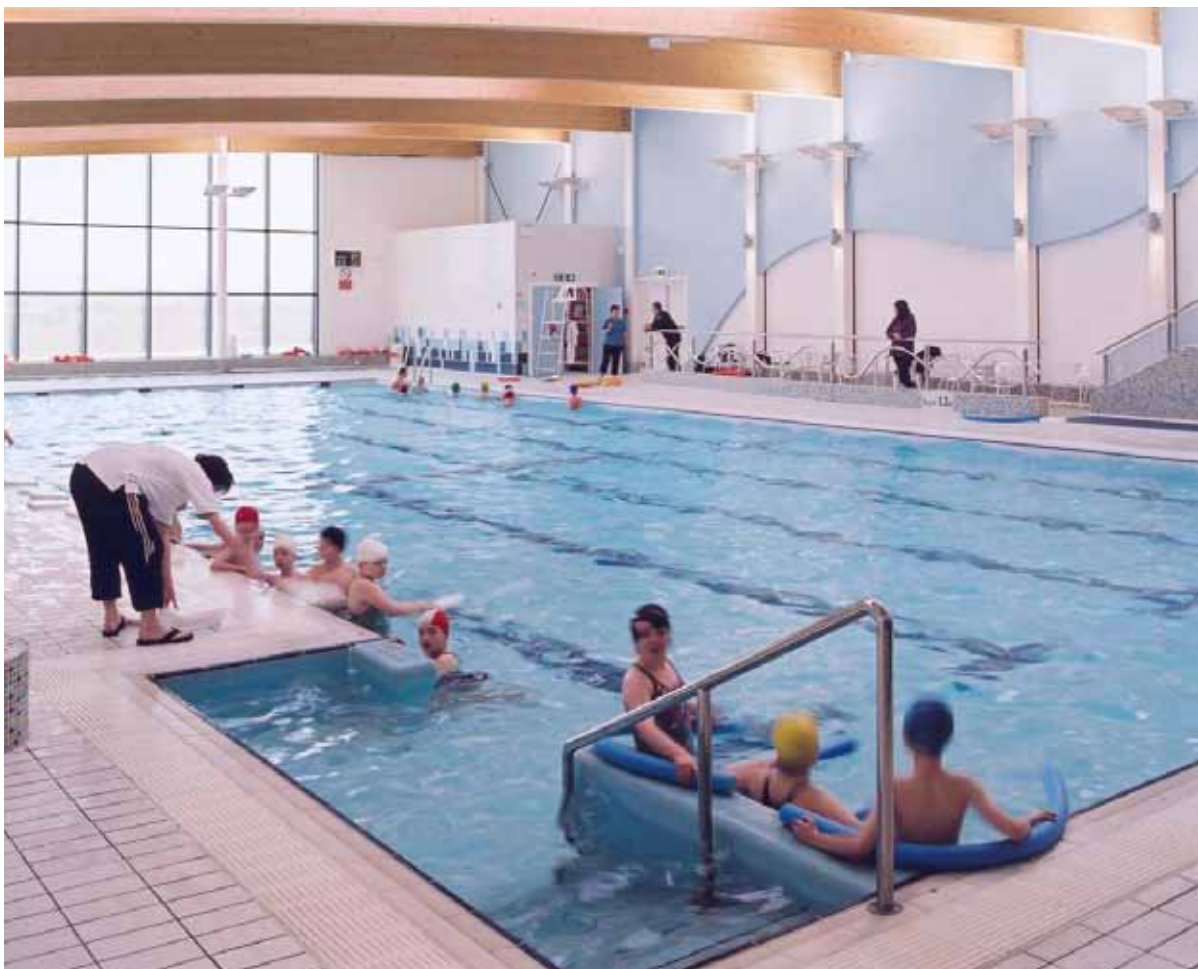
Built-in recessed 'easy going' steps allow safe access to and from the water for ambulant users.
