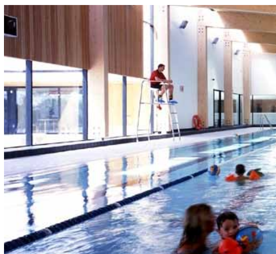
Side lighting can cause specular glare on the pool surface limiting visibility below the water's surface. Careful positioning of lifeguards can minimise the impact of the glare
