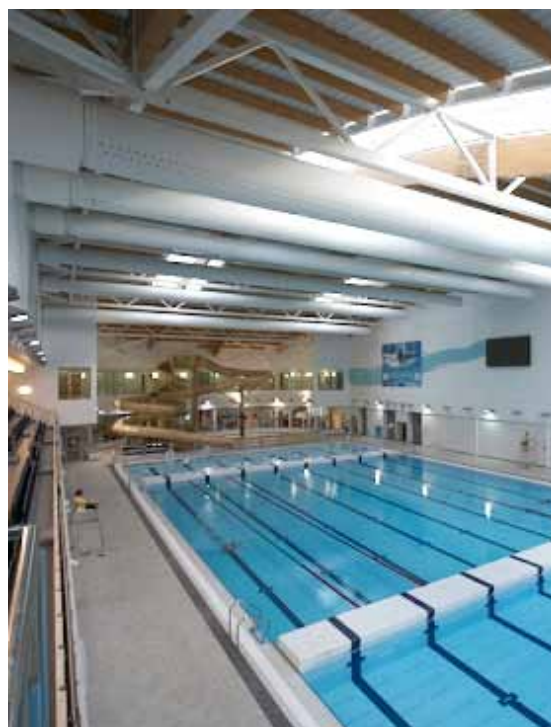
50 m pool divided with two movable bulkheads
