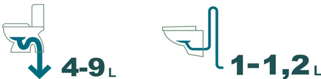
Gravity Toilet – High water usage
