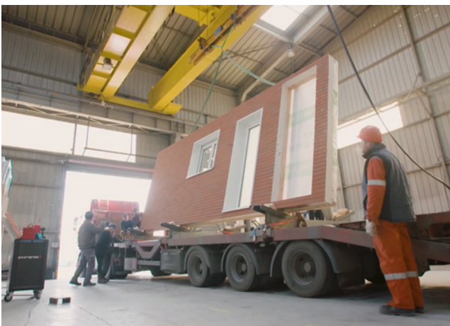
Step 2: Off-site manufacturing: prefabricated facades with triple glazed joinery.
