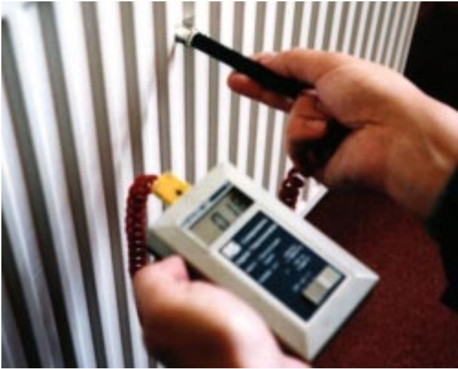
Figure 2 Using a band probe to measure water flow temperature at a radiator
