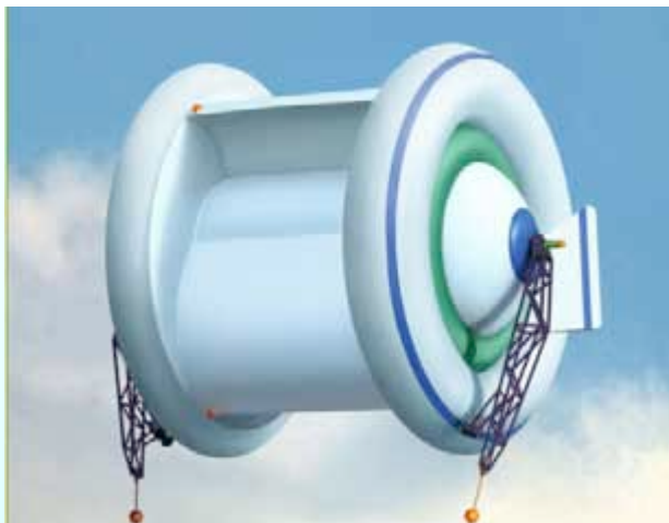
Magenn Power. Helium filled, 150 – 300m high 100kW ~14m by 30m. $500,000. 2010 - 2011
