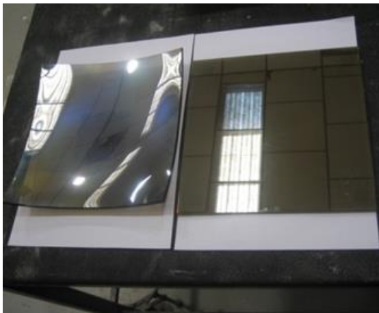
Figure 3.10: Slump formed hot bent glass Coating air side caused colour distortion (Ramboll, 2009).
