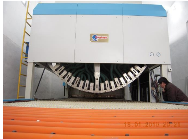
Figure 2.30: Radial curved hot bending equipment allows glass to be tempered. (Xinglass, 2015)
