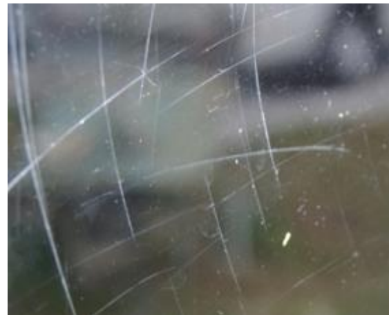
Figure 2.21: Scratches in glass. (Glassworks, 2015)
