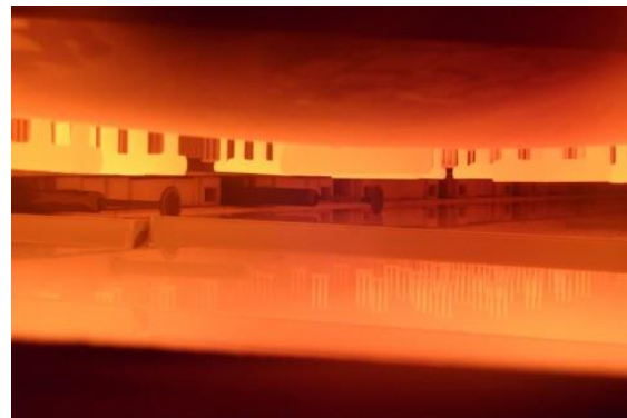
Figure: 2.17: The glass is molten and floated on a tin bath. (Imgbuddy, 2015)
