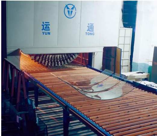
Figure 2.29: Radial curved hot bending equipment allows glass to be tempered. (Glass machinery China, 2015)
