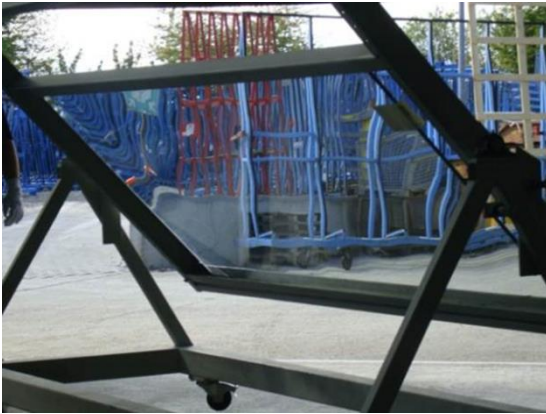
Figure 3.37: Anon project – A typical pane found to have excessive roller wave distortion. (Ramboll, 2013)
