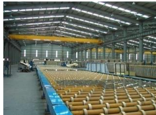
Figure: 2.19: The glass is cut and ready for stacking. (Noval Glass, 2015)
