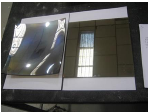
Figure 5.10: Slump formed and flat glass sample – coating air side but distorted. (Ramboll 2009)
