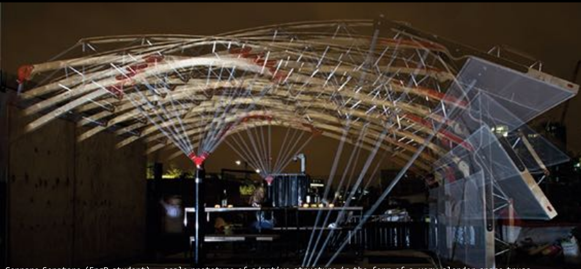
Gennaro Senatore (EngD student) - scale prototype of adaptive structure in the form of a very slender space truss
